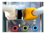
Step 2 Conntet the plug( ) of USB cable to the USB jack of the CID Device hardware.
