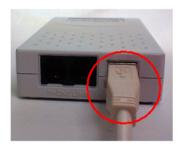
**Step 3** Complete the gateway hardware installation by plugging telephone line and phone line into the two jacks regardless of its location of the gateway hardware.
